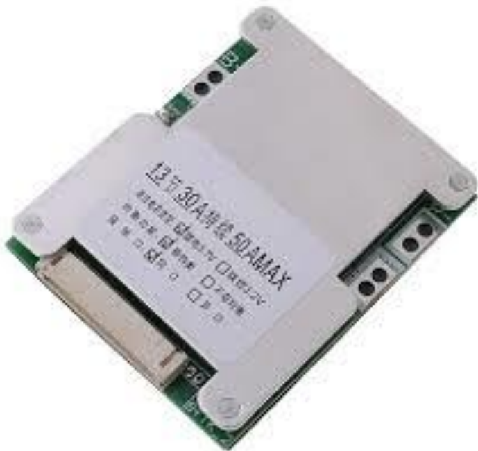
BMS 13S 50A 48V Balanced 18650 Li-ion Lithium Battery Charger Protection Board[/caption]
