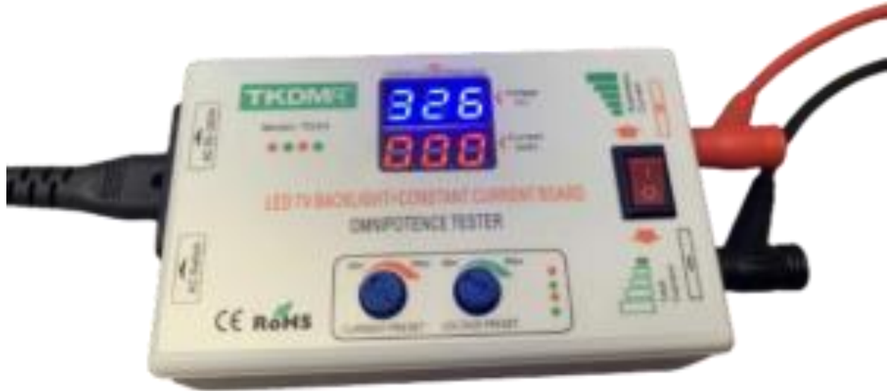
TD3H LED Tester – Voltage, Current, and Electronic Component Measurement[/caption]
