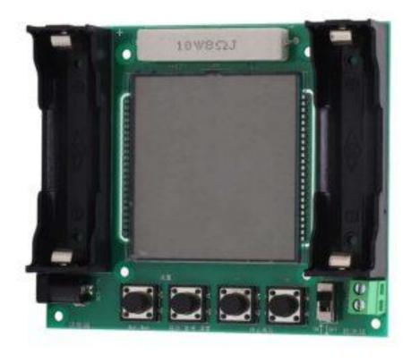
**Key Features of the XH-M239 18650 Battery Capacity Tester with LCD Display**
