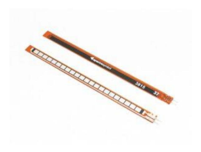
The **Long Flex Sensor** operates as a **variable resistor**. As the sensor bends, its resistance changes proportionally to the degree of flex, allowing microcontrollers to quantify motion or bending angles.
