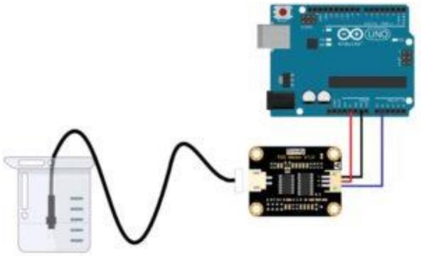
Sensor Meter V1.0 Board Module (Measuring Water Quality)[/caption]
