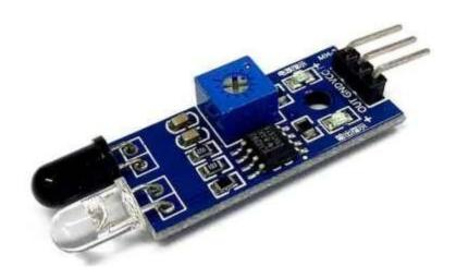
The FC-51 Infrared (IR) Obstacle Avoidance Sensor Board 3-Pin is a compact and reliable sensor module designed for robotics, automation, and electronic projects that require real-time obstacle detection. Utilizing infrared technology, this sensor detects objects in its path without physical contact, making it ideal for line-following robots, collision avoidance systems, automated vehicles, and smart home applications.
