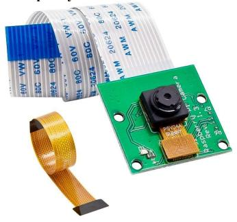
5MP 1080P Raspberry Pi Camera Module Rev 1.3 with Cable
